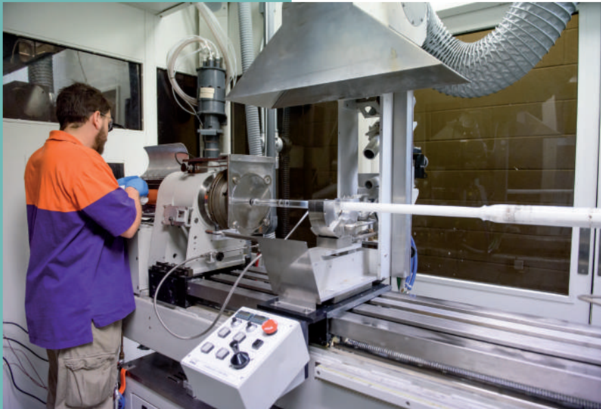
Figure 5.1. The deposition section of a modified chemical vapor deposition (MCVD) lathe. The white glass is the porous silica soot deposited inside of a pure silica substrate tube prior to sintering and consolidation.
