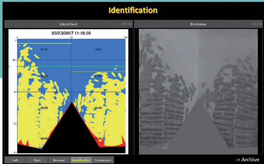
Figure 7.11. Batch coverage converted into a bird's eye view. Source: Glass Service, a.s.
