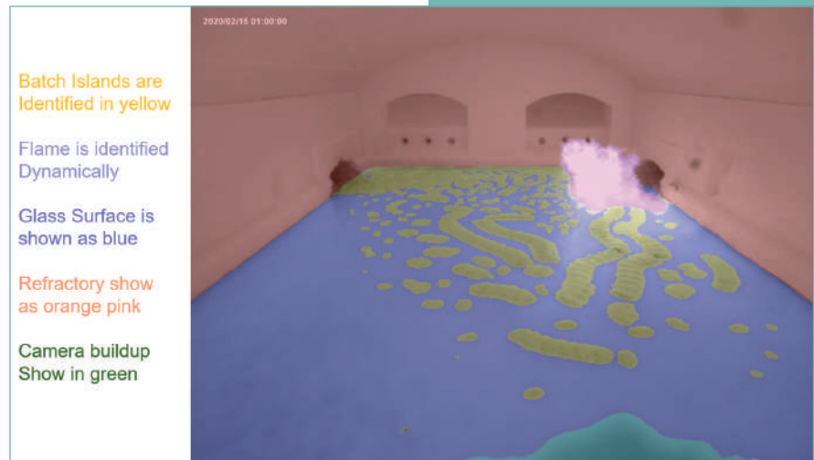
Figure 7.10. Furnace image from a camera identified by a Neural Network. Source: Glass Service, a.s.
