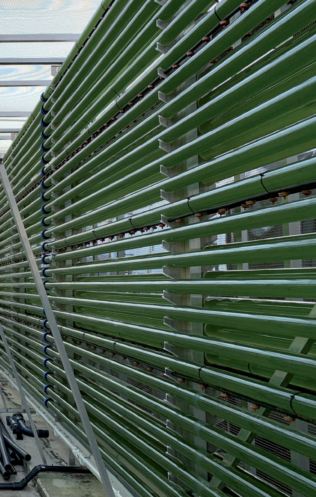
Figure 4.8. A photobioreactor made by Varicon Aqua for microalgae production; tubes are made of borosilicate glass.
