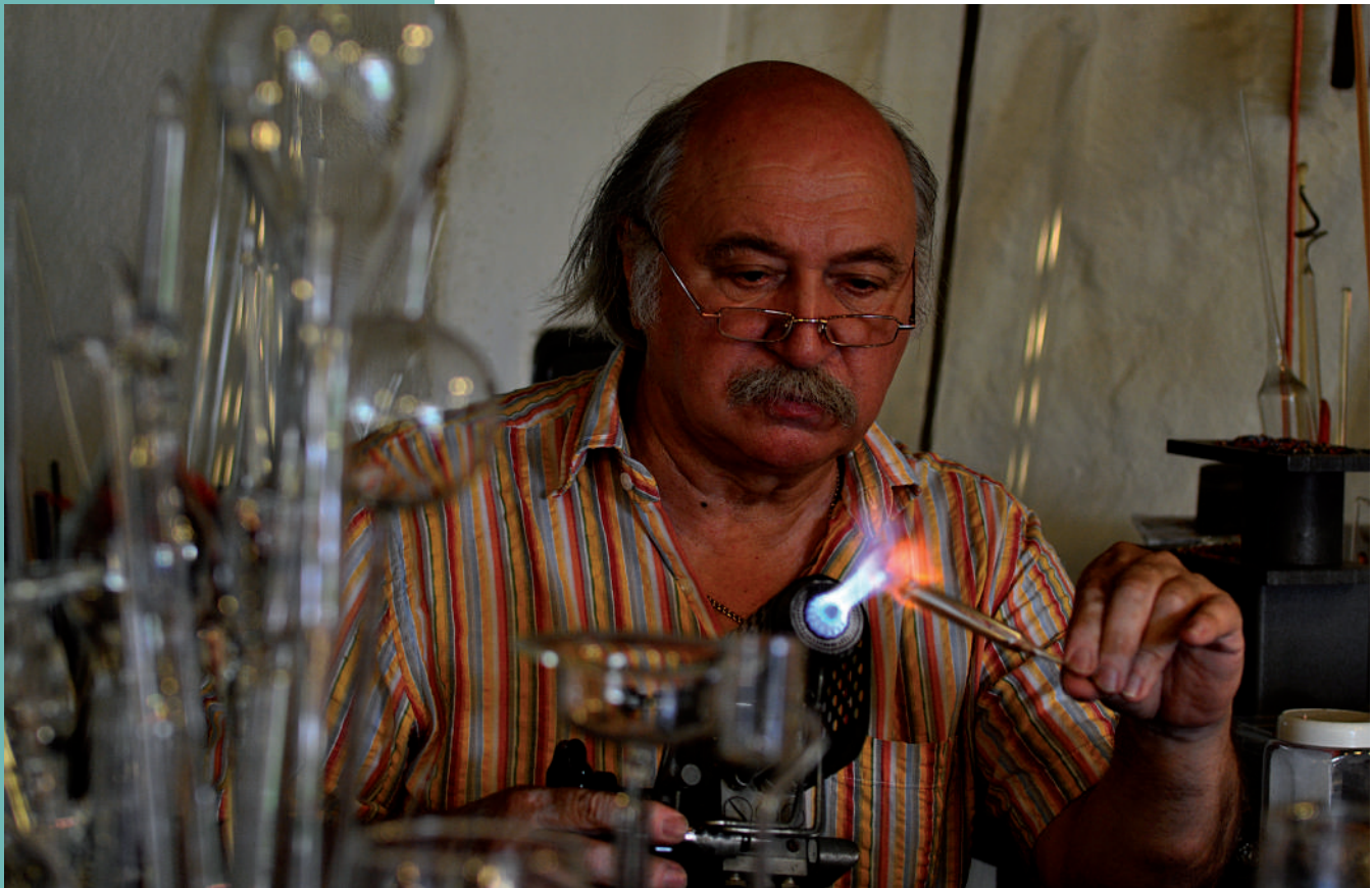
Figure 2.9. Lampworking, used both by the scientific and arts communities for secondary processing.
